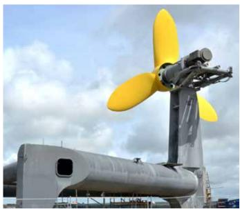
Gravity mounted, direct seawater cooled generator
