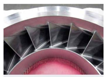
Modifications to the vane geometry would ensure the optimum inlet flow angle which would also improve the mass flow rate (MFR).
