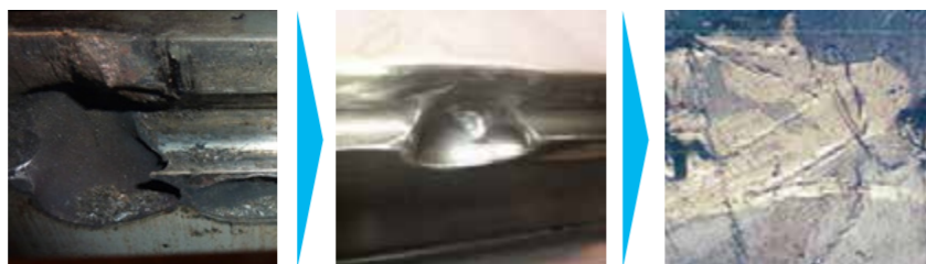
Figure 8. Earth fault location recovery process.
