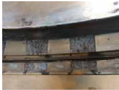
Figure 2. Molten retaining ring fit area.
