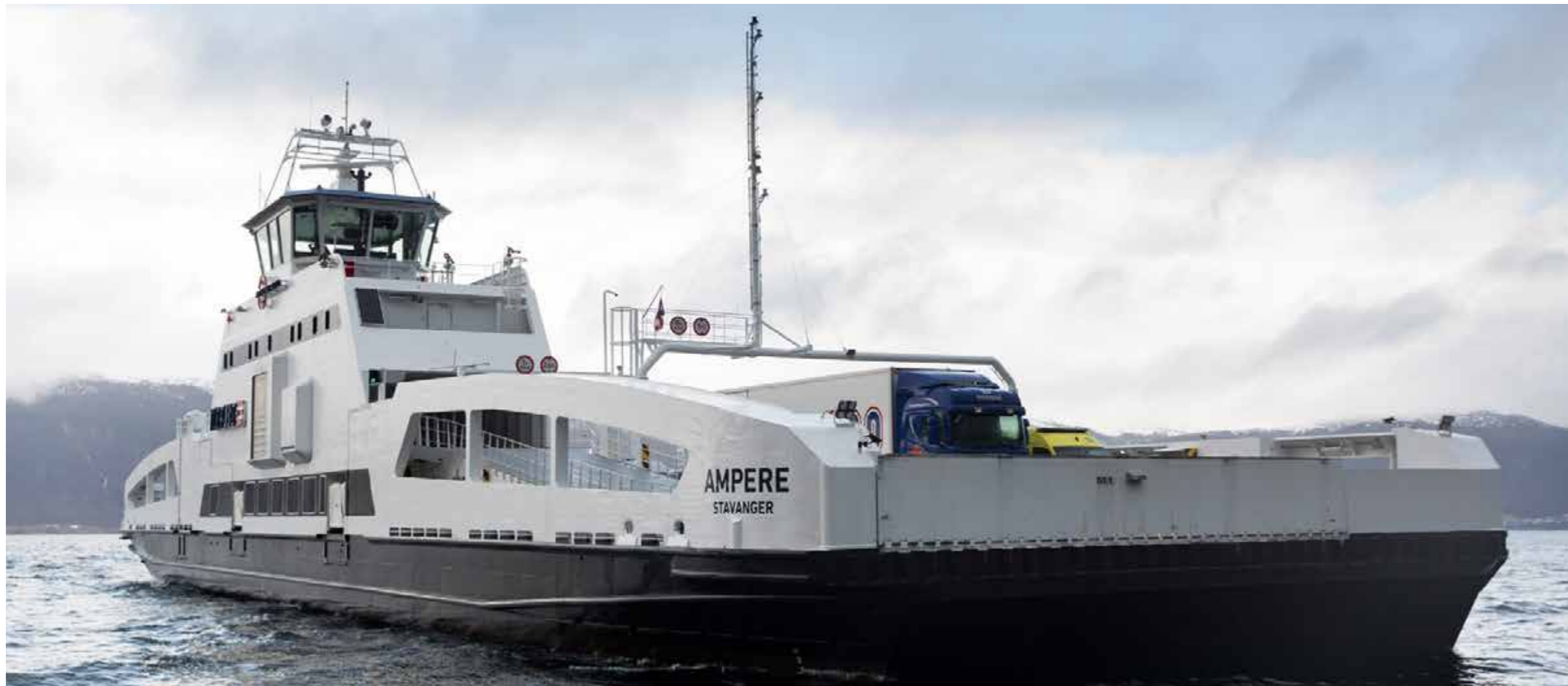
The first electric car and passenger ferry in the world, equipped by Siemens in cooperation with shipbuilder Fjellstrand, has been taken into operation. With three battery packs, one on board and one at each pier, it functions completely emission free.
