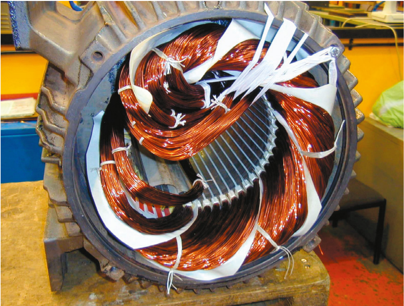
Inserting coils into a 2 pole stator
