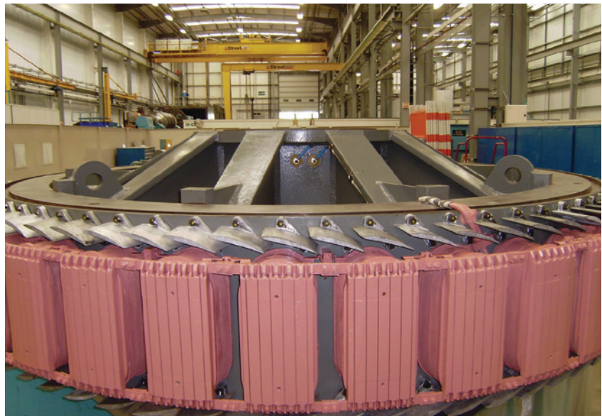
Completed Rotor pictured in the Rugby workshop prior to dispatching and installation on the Mucomir project
