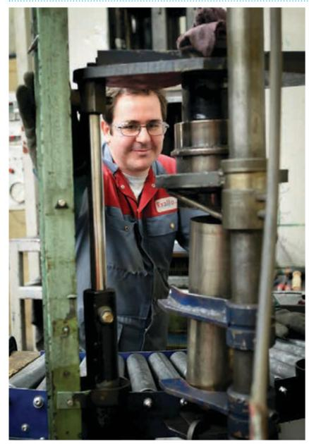
Manufacturing shaft sleeves to protect pump shafts.
