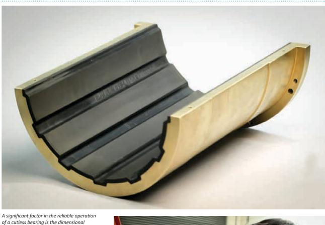
accuracy of the internal rubber lining.
