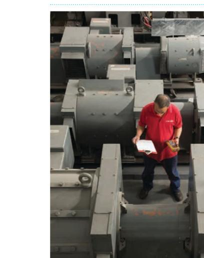
Extensive range of capabilities for testing a wide variety of machines; a sound proofed control room with a state of the art control system and [pictured] the extensive test facility's machine room fed from a 500Vdc 12-pulse rectifier on an 11kV grid supply.
