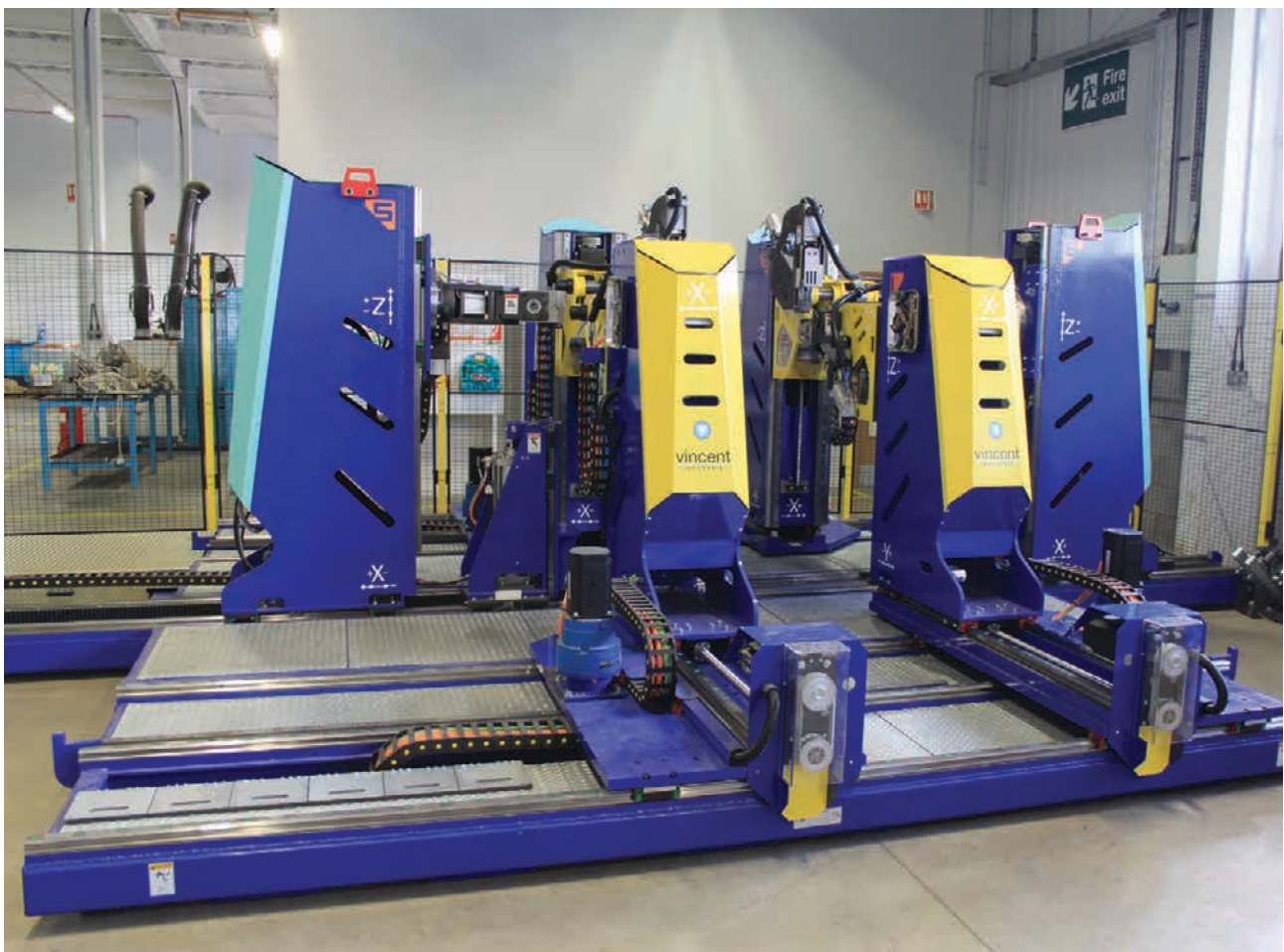
The Vincent Universal Coil and Bar Former to automatically shape the HV coils.
