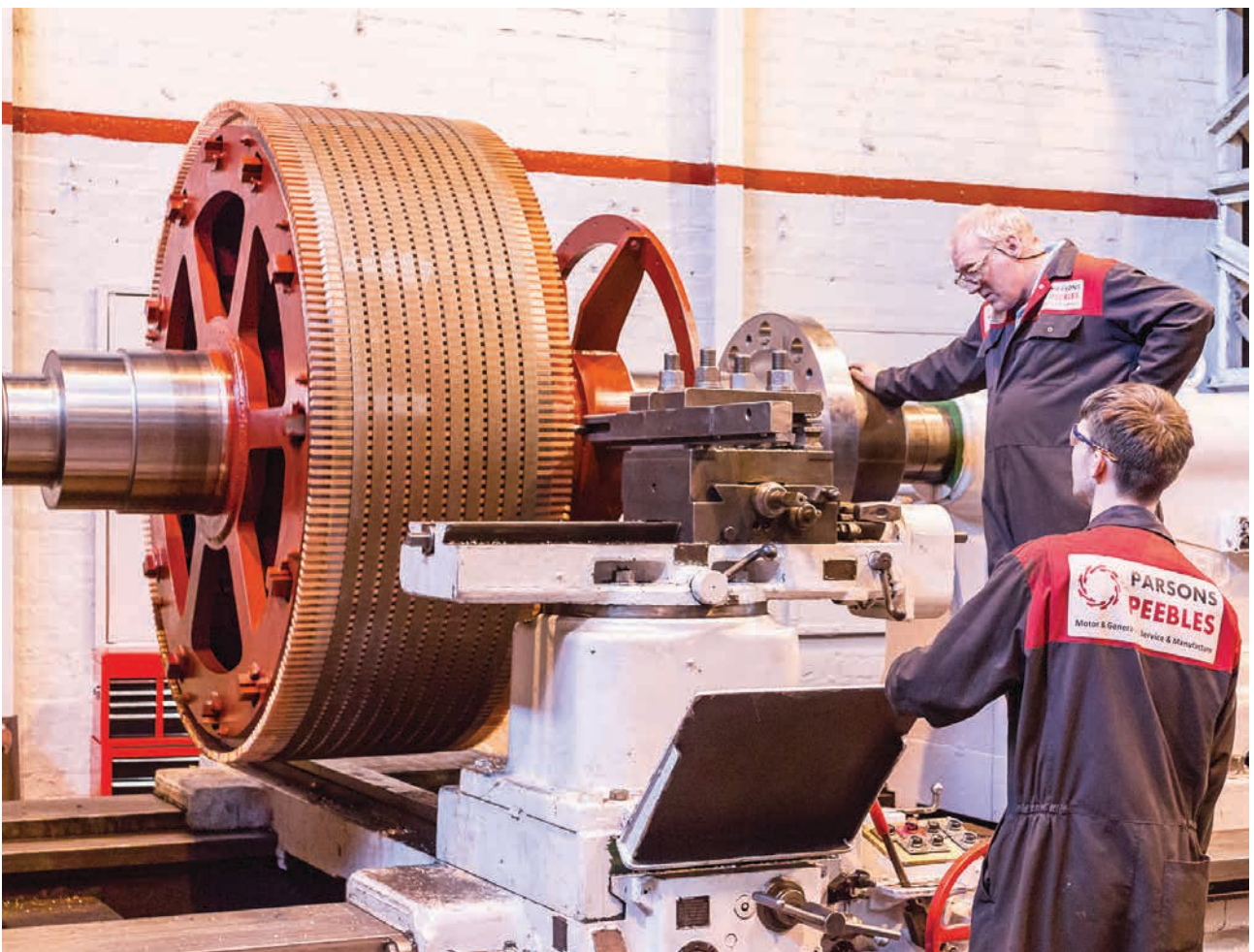
Their 60 tonne Craven lathe capable of handling up to 7 metres in length.
