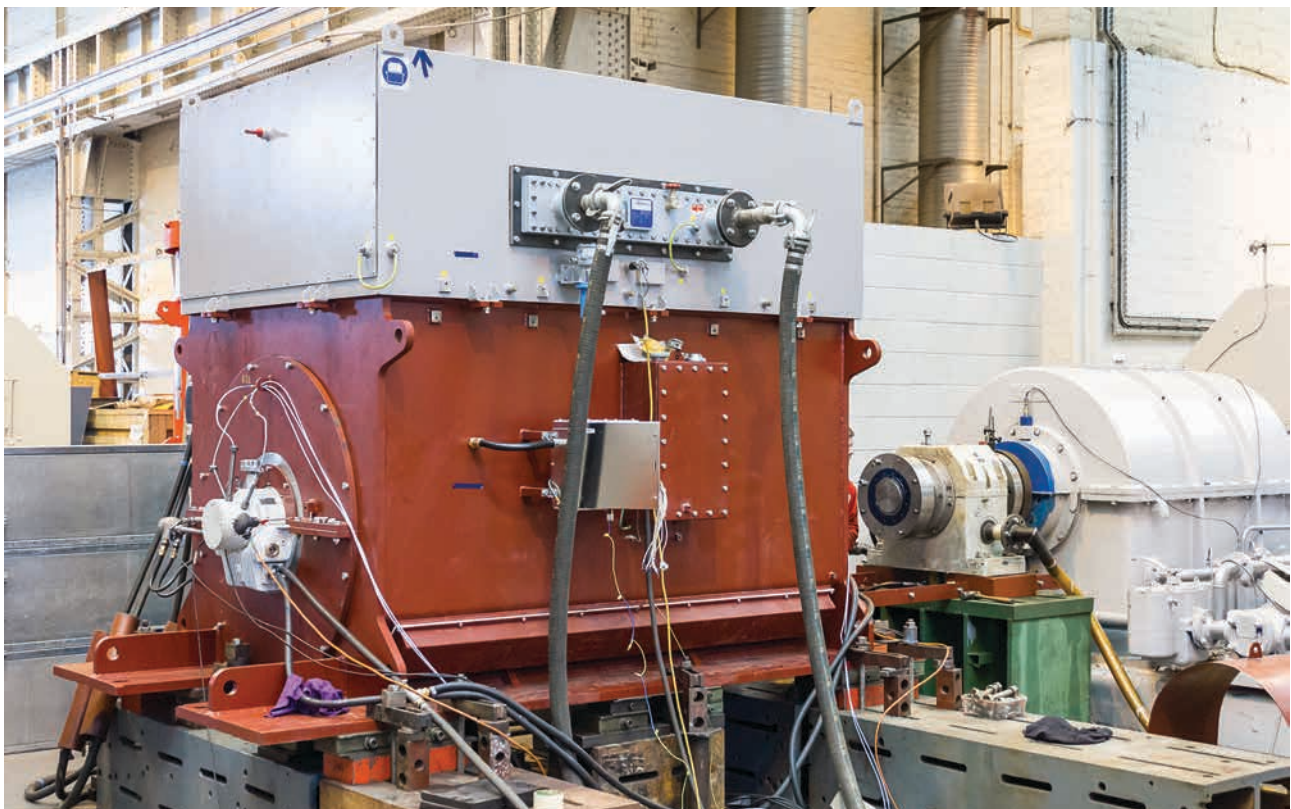
A large machine mounted onto the test bed for a load test.
