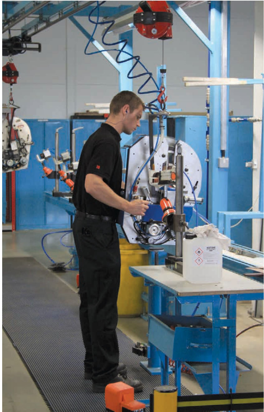
Insulation tape being applied by the semi-automatic Ridgway BCT machines.
