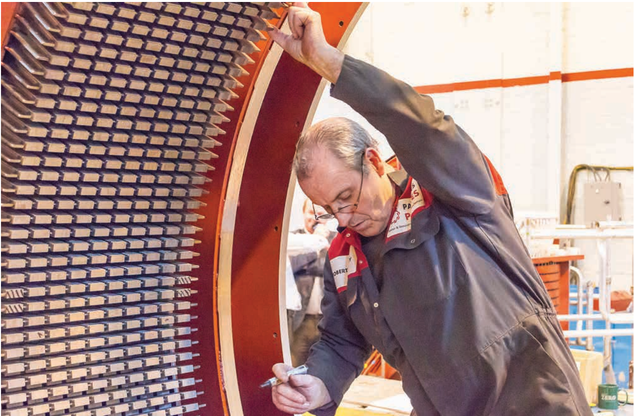
Marking up a new 8 tonne HV stator before inserting the coils.
