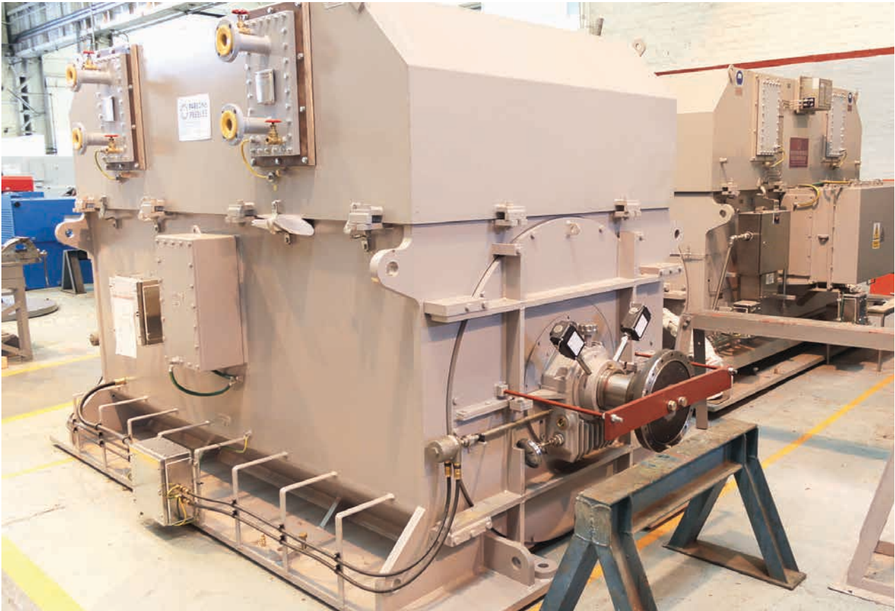
Drop-in replacement motor designed to fit site space envelope and terminal points.
