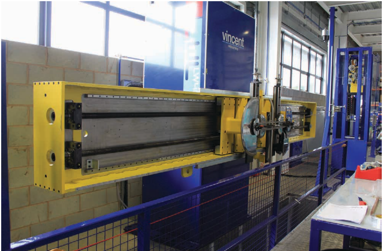
The Vincent 4 metre Coil Loop Winder.
