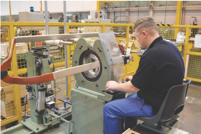
The new coils were redesigned to account for the considerable improvement in insulation technology since the original was manufactured.
