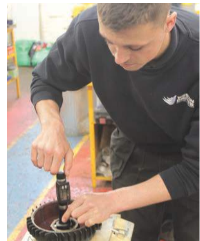
Connor Earnshaw, checking the radial Bearing Housing fit with a three point calibrated micrometre as recommended by SKF.
