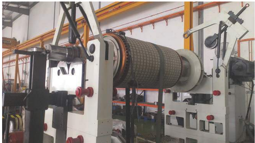
Maser & Quartzelec's 32-ton balancing machine.
