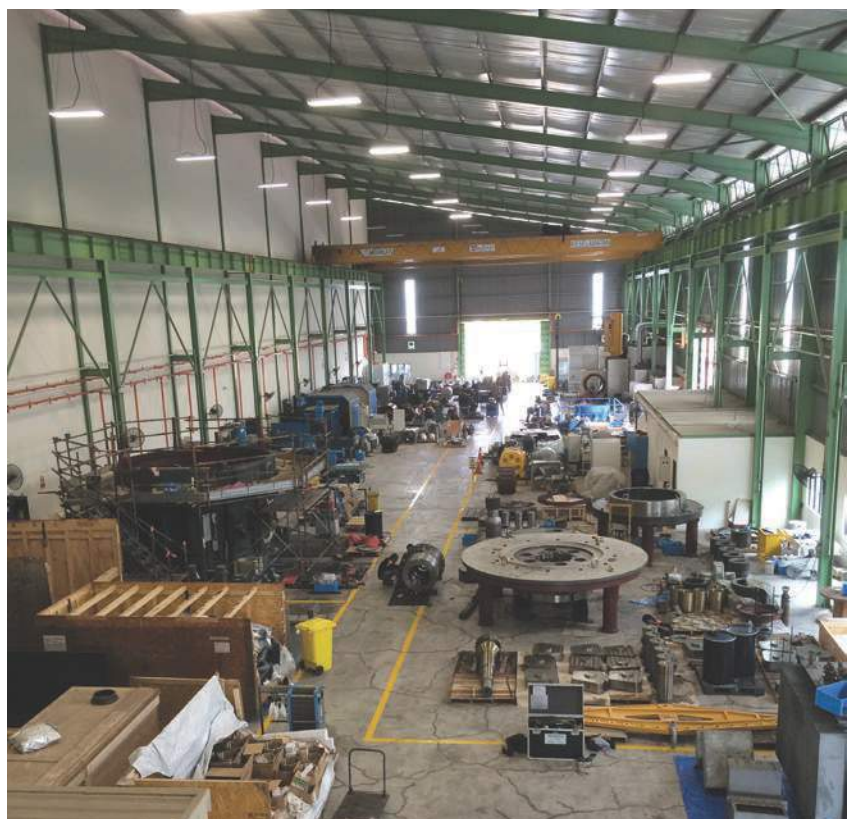
A view down across the new workshop with the Flender gearbox being overhauled in the foreground.
