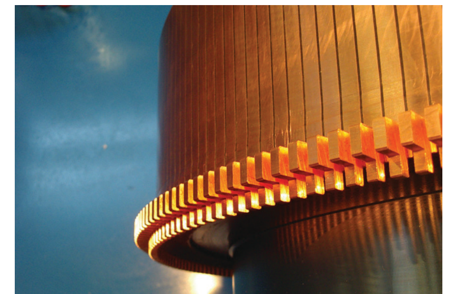
PLD Collettori pride themselves on being one of the only commutator production companies with an inhouse copper drawing machine.
