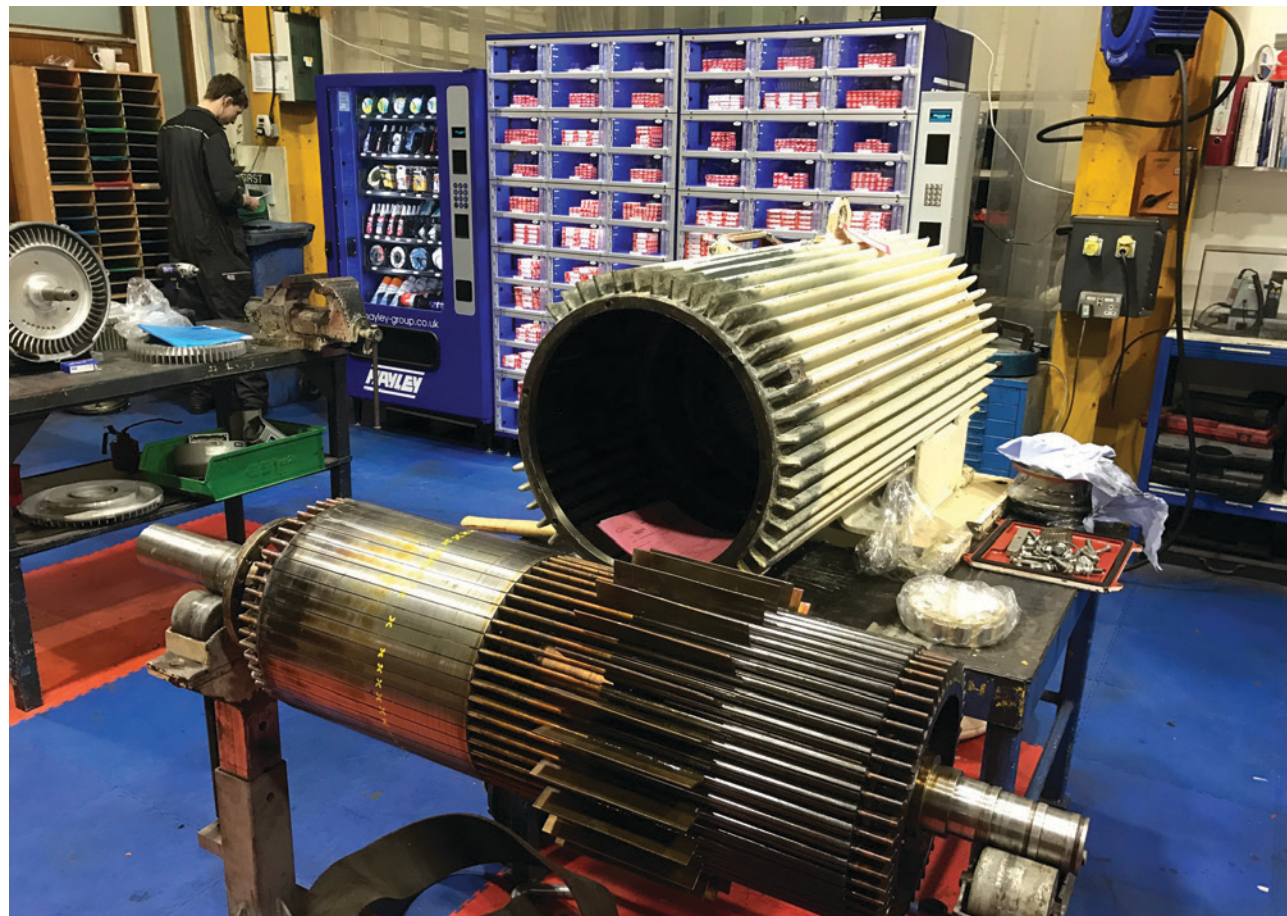
A rare Brook Crompton pipe cage rotor in for repair at Fletcher Moorland.
