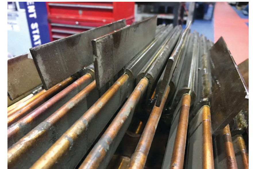
Air agitation fins on the extended cage.
