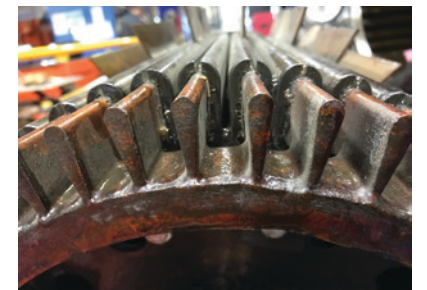
Alloy cladding on the agitation fins.
