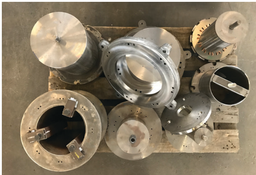
The jigs produced in-house at Nestech ensure tight tolerances are maintained when pressing stacks together.
