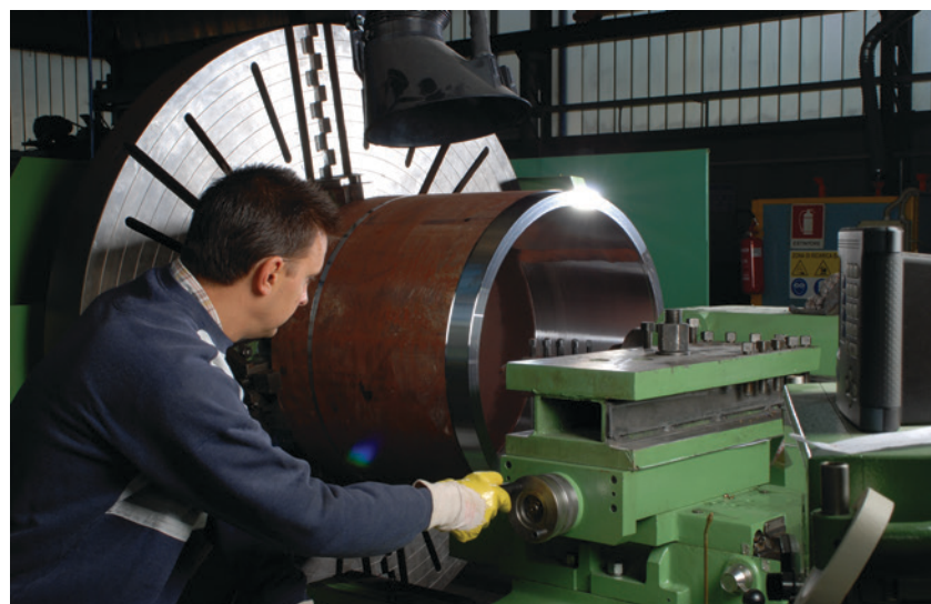
Testing the dimensions of a commutator while machining to size.
