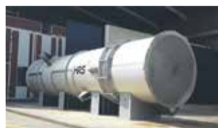
This large gas cooling heat exchanger contains 2,900 separate tubes; a total length of 21km
